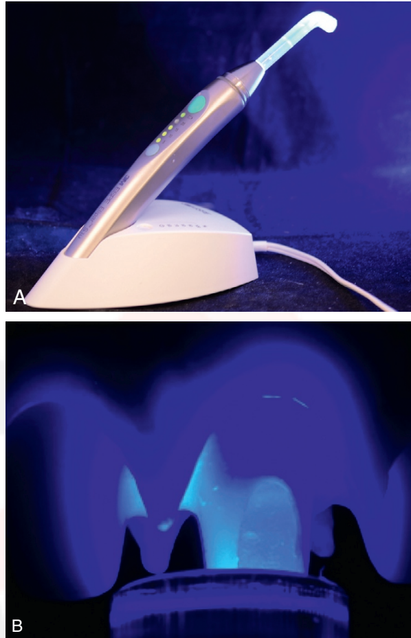
FIG 4-10 Most curing units today are light-emitting diodes (LED) designed (A) to emit high intensity blue light that activates photo-chemicals in the composite, triggering an addition polymerization. The units are generally cordless and have controls for time and, in some cases, intensity. LED units are intense enough to travel through translucent parts of the tooth (B) and bright enough to damage the retina of the eye. Thus, measures to limit visual exposure should be used at all times. (Courtesy Y-W Chen, University of Washington Department of Restorative Dentistry, Seattle, WA.)
